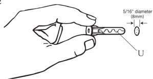
After you have prepared the holes for mounting the Wall Plate (WP), install the wall plate by inserting the four (or six) Lag Bolts (T) through the mount and into the ALLIGATOR $^*$  Anchors (U) as shown in Figures 10 and 13. After checking that the wall mount is level, tighten all lag bolts fully, but be careful not to over-tighten.
